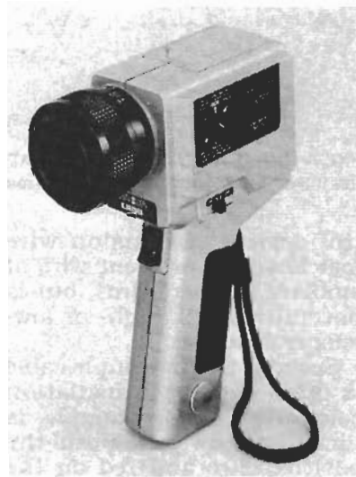
FIG. 9—THIS HANDHELD DEVICE measures temperature using noncontact infrared, radiation thermometry.
