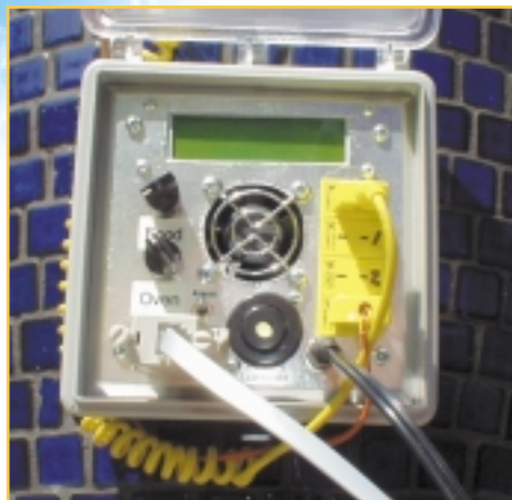
Photo 2: The LCD shows the actual and desired cooker temperatures, and up to three food temperatures. You can mute the piezoelectric alarm. The cooker temperature can be set from 180° to 400°F in 5° steps, and the food alarm can be set from 100° to 220°F.
