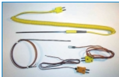
Photo 3: Beaded-type thermocouples respond too quickly for use in an oven. Adding a washer provides thermal mass. The slender stainless probes are used for food temperatures. The thicker probe is for oven temperatures.
