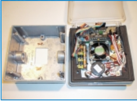
Photo 6: The electronics are assembled on a piece of double-plane prototype board and mounted over the LCD. The weatherproof gasket and cover come with the electrical box.
