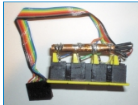
Photo 4: An LM34 (inside the 0.25 inch copper tube) measures the tube's temperature, which is approximately isothermal with the thermocouple connector.
