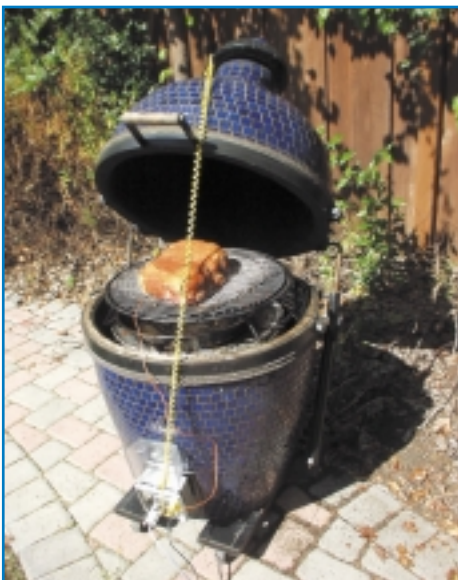
Photo 7: A typical setup includes food, oven and food temperature probes, and the controller.
