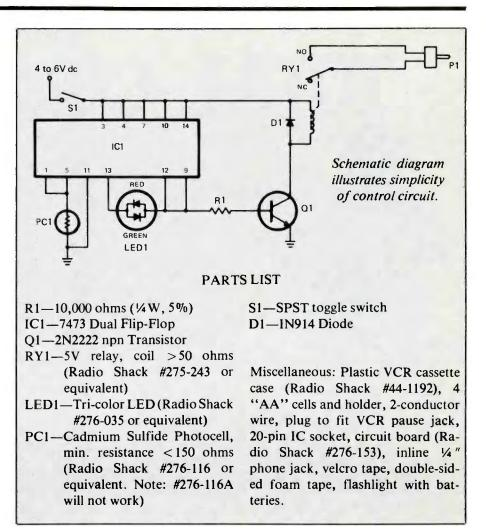
well-lighted room, it should be recessed about an inch back inside the case. The barrel of an inline phone jack, fitted through the case opening and over the photocell, assures proper alignment and provides a finished appearance. The circuit board can be attached to the case with velcro tape, allowing for easy repositioning, while the battery holder can be fastened with double-stick foam tape. Any two-conductor wire may be used to connect plug P1.
