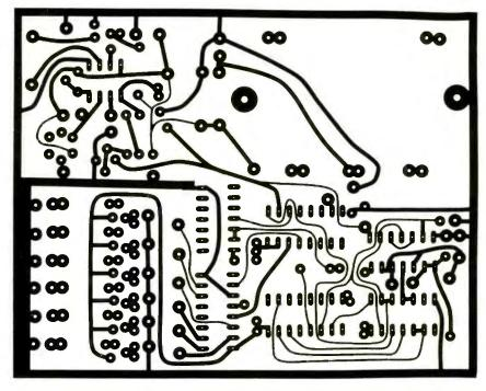
*Fig. 8. Actual-size etching-and-drilling guide for receiver/decoder pc board.*
