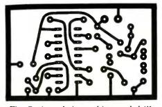
Fig. 7. Actual-size etching-and-drilling guide for transmitter pc board.
