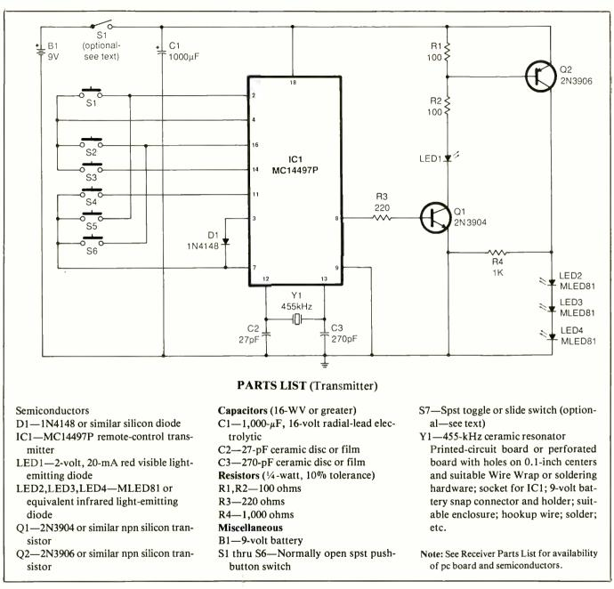
Fig. 1. Complete schematic diagram of transmitter circuit.
