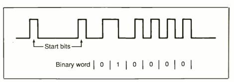
Fig. 2. Binary word for channel A is 000010, which indicates that all bits are 0 except one, which has a binary weight of 2.
