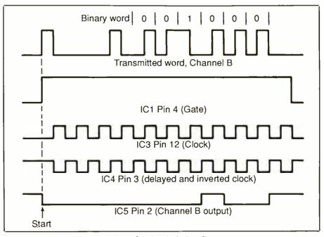
Fig. 6. Decoder circuit timing diagram.
