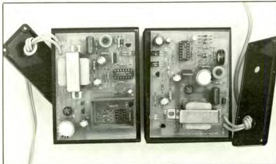
Fig. 13. Photo shows fully wired transmitter (left) and receiver (right) circuit-board assemblies just prior to installation in the enclosures atop which they sit.
