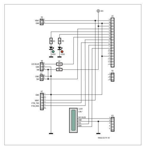
Figure 4. LoRa Button schematic. This is the 'sending' or 'master' part of the Elektor LoRa Node. The OLED display is optional and its use requires deep thought about energy use!
