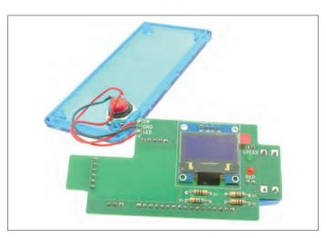
Figure 9. The almost completed LoRa Button board.
