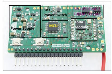
Figure 1. The LoRa Node control board with 'real estate' allocated to functional blocks. Actually, you are looking at a minimally-stuffed LoRaWAN Node Experimental Platform.
