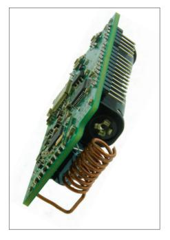
Figure 10. The feedpoint of the home-wound, quarter-wave antenna for the 868-MHz band is soldered to the ANT pad on the LoRa Button board (early prototype shown). Note the coiled construction of the antenna.
