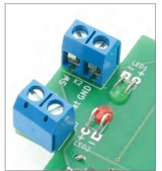
Figure 5. A special method for mounting the LEDs is applied on the LoRa Button board.
