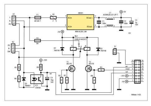
Figure 11. Schematic of the LoRa AC Switch. This is not a 'dumb' device but it feeds the actual relay on/off state back to the LoRa Node.
