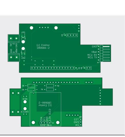
K3 employs only seven of the sixteen pins on this PCB. It has two options as discussed below but both assume the LoRa Node board has a standard 0.1-inch pitched, angled connector in position K5. The seven pins in positions 11 through 17 (see board 180516-1) are enough, but K3 can also be a 17-pin pinheader (cut to length) over the full length of K5.
