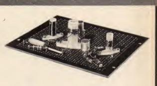
L2/3 an Aladdin former with dust core. L3 wound first—9½ turns 28 s.w.g. enam. wire close wound. L2 2 turns 28 s.w.g. enam. wire wound on top of L3 at "TRI collector" end
