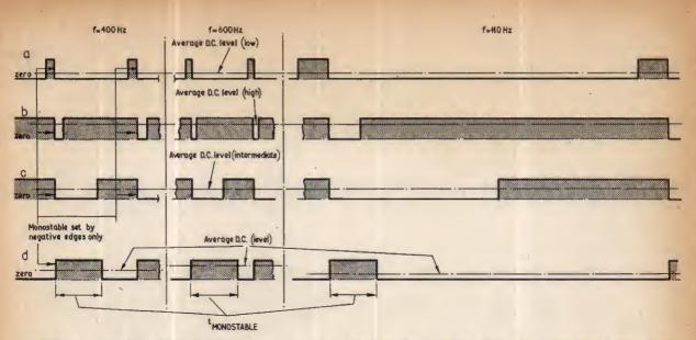
(a) Steering control waveforms PortRudder (b) Steering control waveforms Starboard (c) Steering control waveforms Rudder (d) Corresponding Throttle control waveforms Amidships
