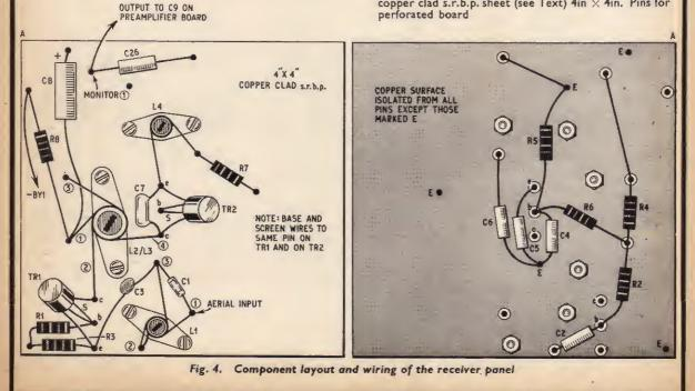
Because of the fact that TR2 operates very close to its cut-off point, its characteristic is non-linear, and it is this non-linearity which provides the essential characteristic for detection of the modulation of the carrier. Therefore, TR2 performs the dual role of high gain r.f. amplifier and detector.
