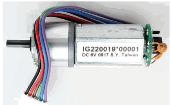
Photo 3. This Diligent gear motor interfaces directly to the motor shield via J3 or J6. A pair of Hall-effect sensors produces a quadrature signal as the motor shaft rotates.
