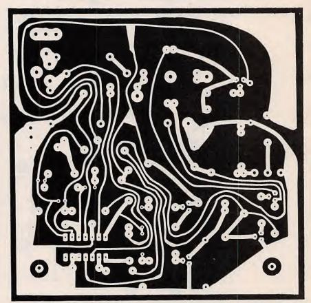
Fig. 3. Actual-size etching and drilling guide for a printed-circuit board for the controller is shown above. Component layout is at top. Note that there are sevral different options regarding components and construction, as outlined in text and Parts List. C3 to the +9-volt line by replacing R6 with a jumper. The *IC1C* output signal is coupled through R18 to the Q3 input, in parallel with the ramp from C10.
