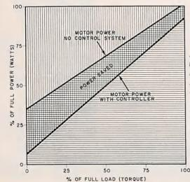
Fig. 1. These curves are the results of tests made by NASA on a ½-hp split-phase and ¼- and ¾-hp capacitor-start motors. Note that the power-factor controller reduced the no-load power demand by a factor of 6. Motor slowdown was less than 2%.
