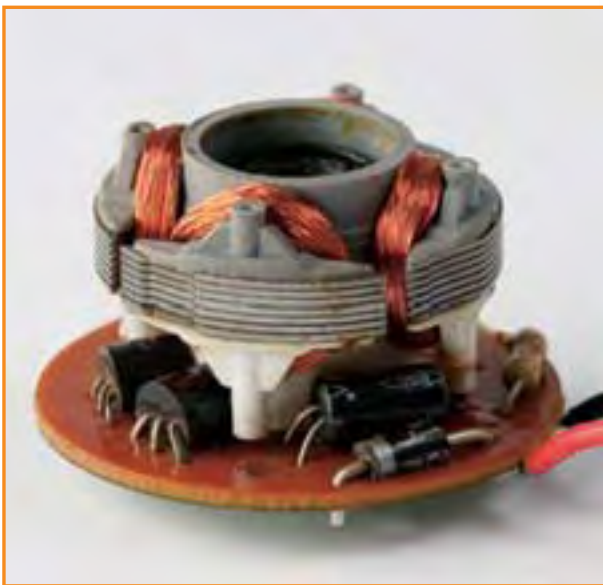
Figure 3. For a comparison we opened up an older fan. The drive electronics and sensor are all discrete components.
