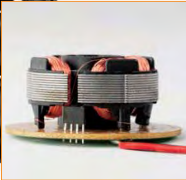
Figure 2. Calling it a rotating magnetic field generator seems to be an overstatement: all the electronics and the Hall sensor are in a 4-pin IC. Apart from an electrolytic capacitor no other components are required.
