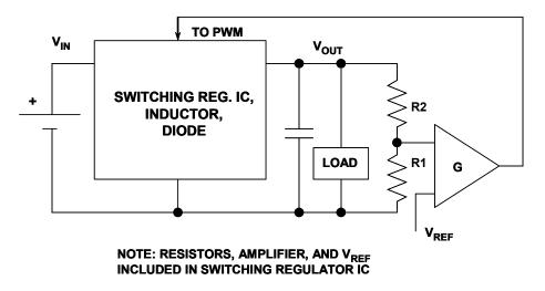
Figure 9.37: Voltage Feedback for PWM Control
