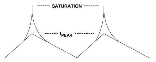
Figure 9.52: Effects of Saturation on Inductor Current
