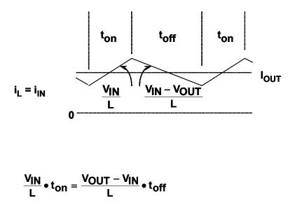
$$V_{OUT} = V_{IN} \bullet \frac{t_{On} + t_{Off}}{t_{Off}} = V_{IN} \bullet \frac{1}{1 - D}$$
