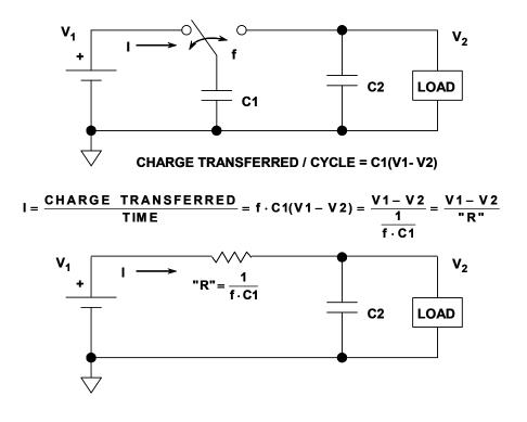
Figure 9.69: Continuous Switching, Steady State
