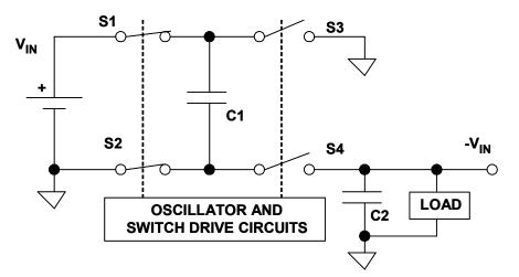
Figure 9.70: Switched Capacitor Voltage Inverter
