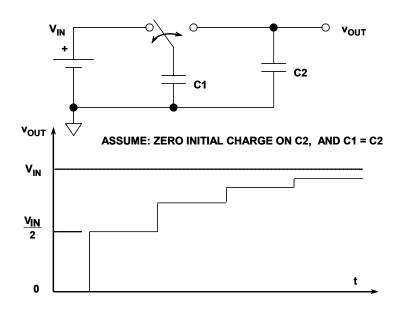
Figure 9.68: Continuous Switching
