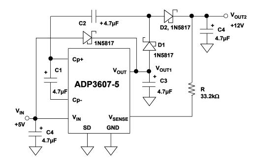
Figure 9.79: Regulated +12 V from a +5 V Input
