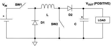
The Absolute Value of the Output Can Be Less Than Or Greater Than the Absolute Value of the Input
