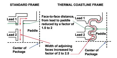
Figure 9.13: Details of the Thermal Coastline Package
