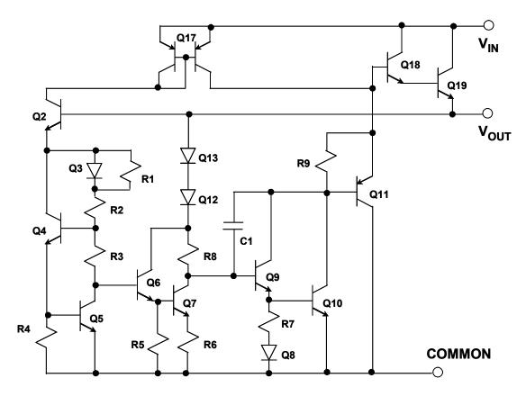
*Figure 9.5:* Simplified Schematic of a LM309 Fixed 5 V/1 A Three Terminal Regulator
