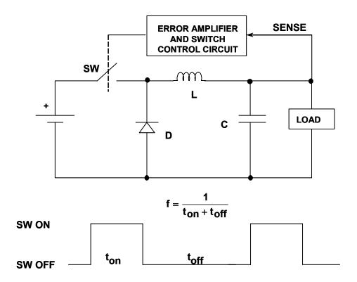
Figure 9.19: Basic Step-down (Buck) Converter
