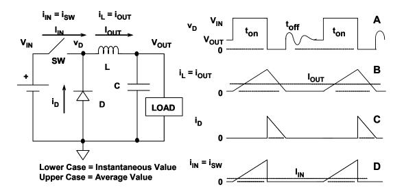
Figure 9.21: Input/Output Relationships for a Buck Converter
