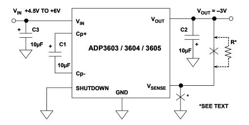
**Figure 9.77:** ADP3603/ADP3604/ADP3605 Application Circuit for -3 V Operation
