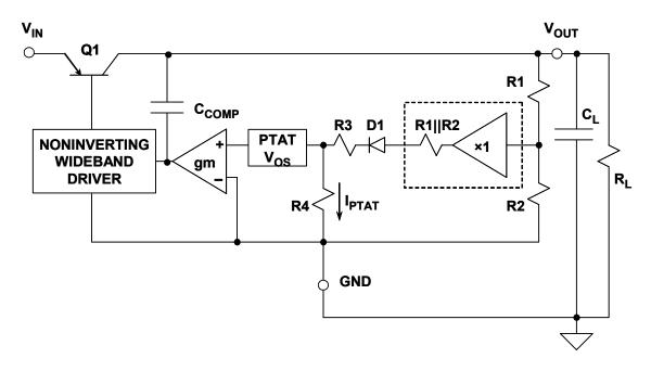
*Figure 9.9:* ADP330X anyCAP Topology Features Improved DC and AC Performance over Traditional LDOs
