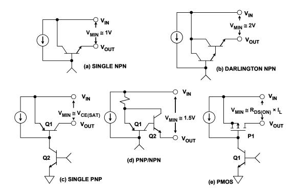
Figure 9.3: Pass Devices Useful in Voltage Regulators
