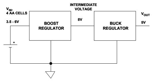
Figure 9.32: Cascaded Buck Boost Regulators (Example Voltages)
