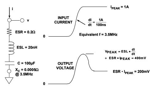
Figure 9.56: Response of a Capacitor to a Current Step
