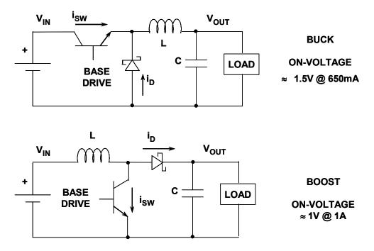
Figure 9.41: NPN Switches in IC Regulators
