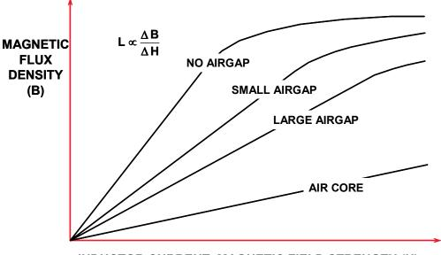
INDUCTOR CURRENT, MAGNETIC FIELD STRENGTH (H)
