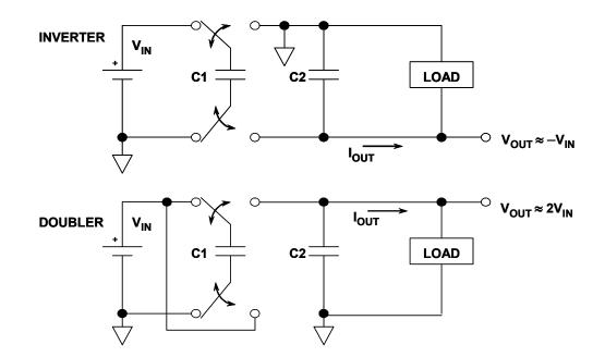
Figure 9.63: Basic Switched Capacitor Voltage Inverter and Doubler
