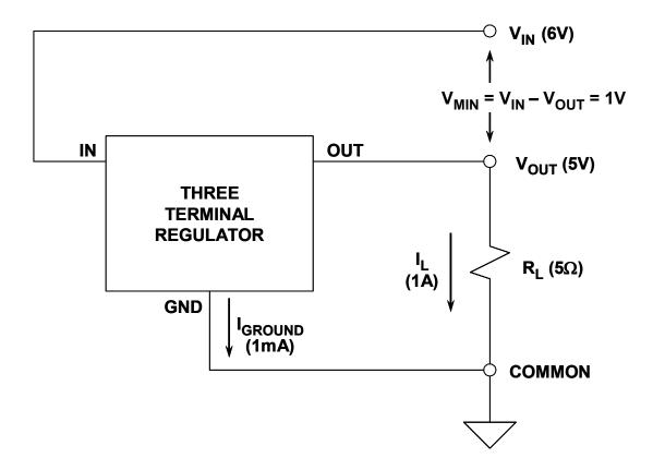
Figure 9.1: A Basic Three Terminal Voltage Regulator
