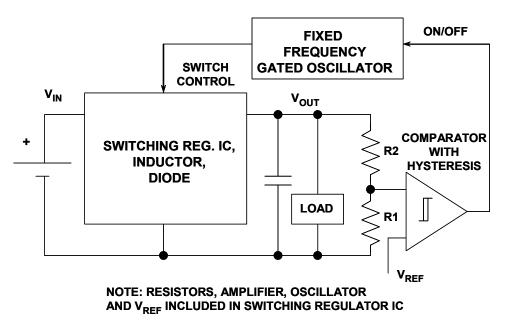
Figure 9.39: Switch Control Using Gated Oscillator (Pulse Burst Modulation, PBM)
