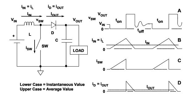
Figure 9.27: Boost Converter Waveform—Discontinuous Mode
