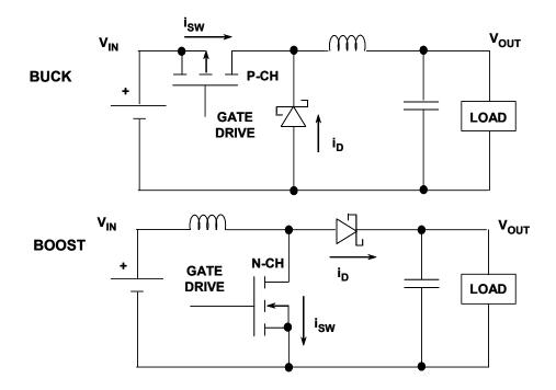
Figure 9.43: Power MOSFET Switches
