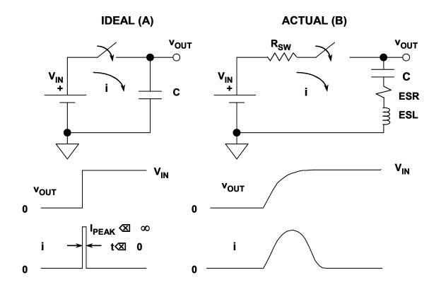
Figure 9.66: Charging a Capacitor from a Voltage Source
