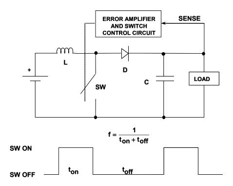
Figure 9.24: Basic Step-Up (Boost) Converter
