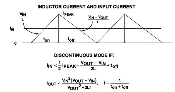
Figure 9.28: Boost Converter Point of Discontinuous Operation
