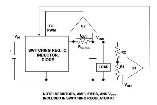
Figure 9.38: Current Feedback for PWM Control
