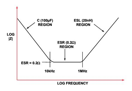
Figure 9.57: Typical Electrolytic Capacitor Impedance vs. Frequency
