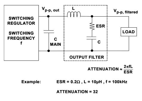
Figure 9.61: Switching Regulator Output Filtering
