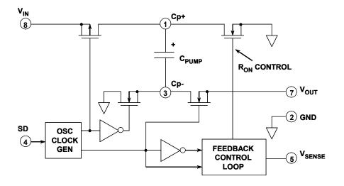
Figure 9.76: ADP3603/ADP3604/ ADP3605 Regulated -3 V Output Voltage Inverters
