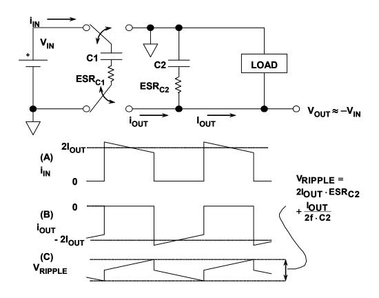
Figure 9.72: Voltage Inverter Waveforms
