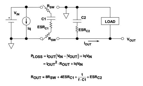
Figure 9.74: Voltage Inverter Power Losses
