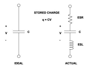
Figure 9.65: Stored Charge in a Capacitor
