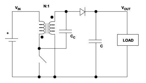
Figure 9.33: Single-Ended Primary Inductance Converter (SEPIC)
