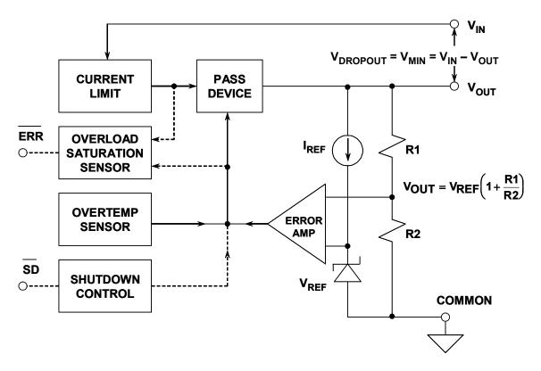
Figure 9.2: Block Diagram of a Voltage Regulator
