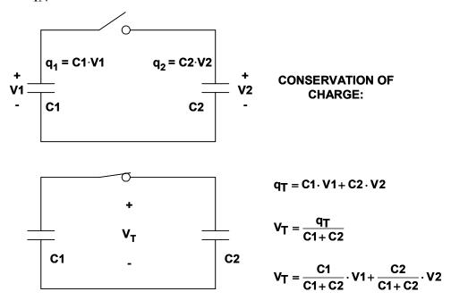
Figure 9.67: Charge Redistribution Between Capacitors
