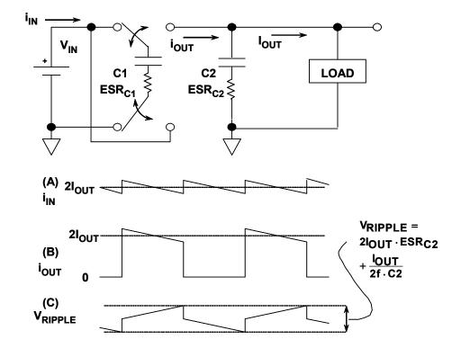
Figure 9.73: Voltage Doubler Waveforms
