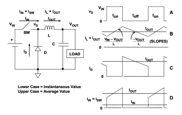
Figure 9.20: Basic Step-Down (Buck) Converter Waveforms
