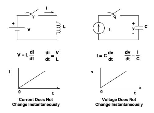
Figure 9.18: Energy Transfer Using an Inductor
