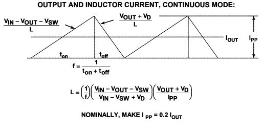
*Figure 9.48:* Calculating L for a Buck Converter: Constant Frequency PWM Type
