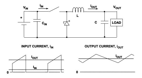
Figure 9.54: Buck Converter Input and Output Current Waveforms
