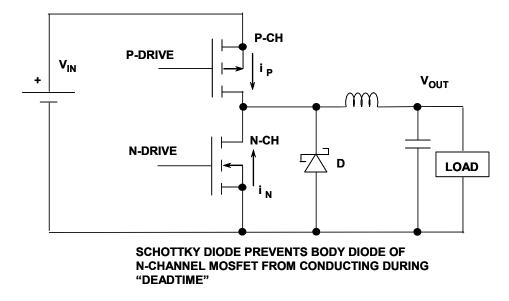
Figure 9.44: Buck Converter with Synchronous Switch Using P- and N-Channel MOSFETS
