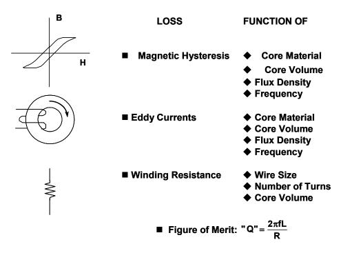
Figure 9.53: Inductor Power Losses
