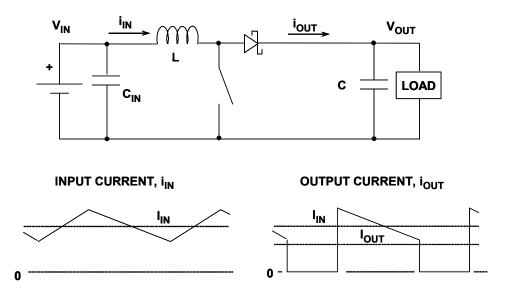
Figure 9.55: Boost Converter Input and Output Current Waveforms
