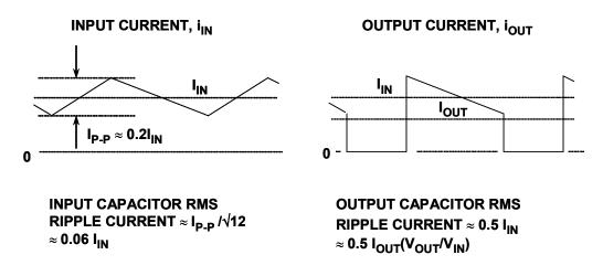
*Figure 9.60:* Boost Converter Input and Output Capacitor RMS Ripple Current Approximations
