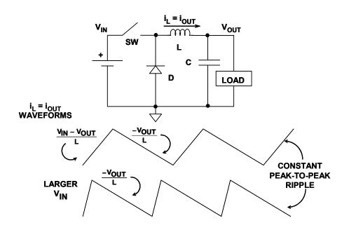
*Figure 9.36:* Control of a Buck Converter using Fixed Off-Time, Variable Frequency PWM
