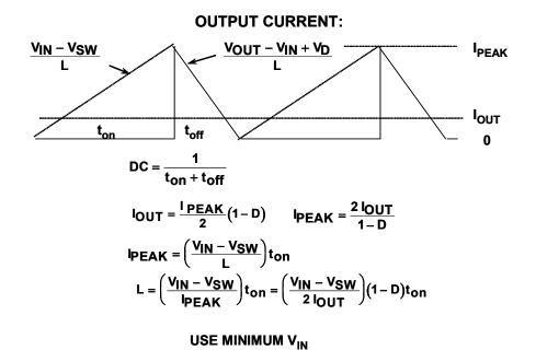
Figure 9.47: Calculating L for a Boost Converter: Gated Oscillator (PBM) Type
