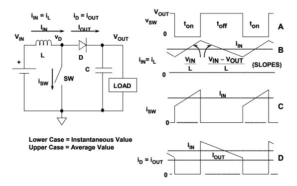
Figure 9.25: Basic Step-Up Converter Waveforms
