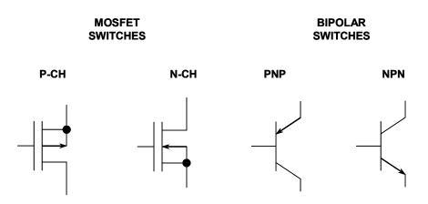
Figure 9.71: Switches Used in Voltage Converters
