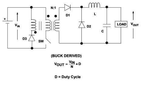
Figure 9.35: Isolated Topology: Forward Converter
