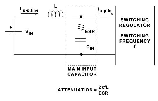
Figure 9.62: Switching Regulator Input Filtering
