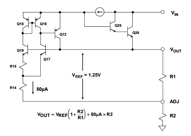
$$V_{OUT} = V_{REF} \left( 1 + \frac{R2}{R1} \right) + 50 \mu A \times R2.$$
