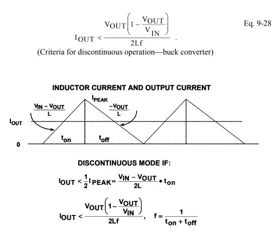
Figure 9.23: Buck Converter Point of Discontinuous Operation
