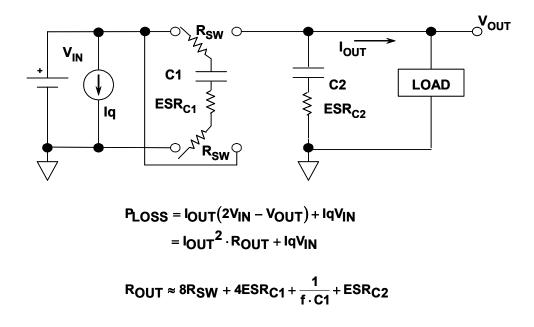
Figure 9.75: Voltage Doubler Power Losses
