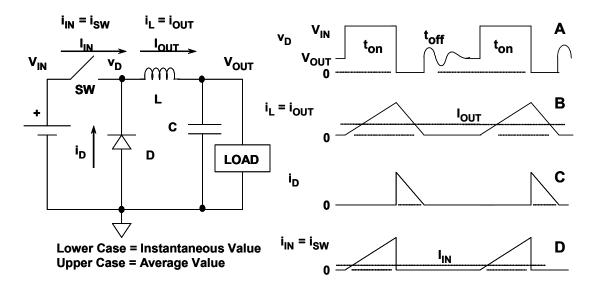
Figure 9.22: Buck Converter Waveforms— Discontinuous Mode
