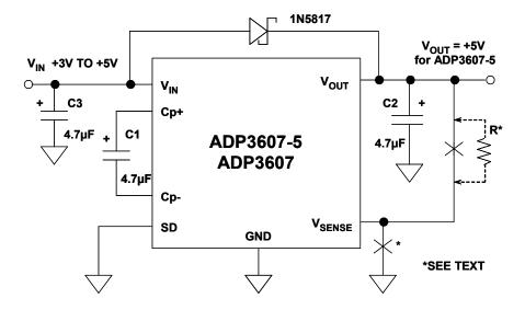
Figure 9.78: ADP3607 Application Circuit
