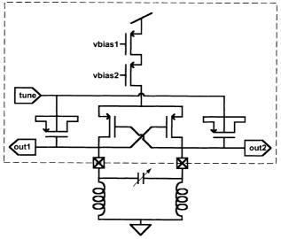
Fig.7. Schematic of the LC VCO.
