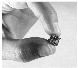
Fig.5. The complete miniature FM receiver module.
