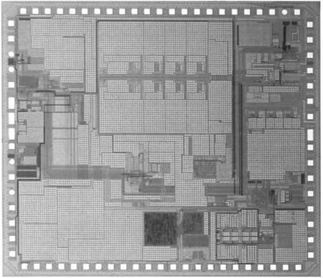
Fig.12. Microphotograph of the FM receiver.
