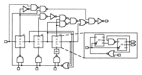
Fig.11. Improved PSRR design of a prescaler.
