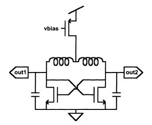
Fig.2. Basic topology of a differential LC oscillator.
