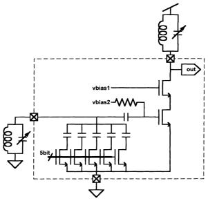
Fig.6. Schematic of the LNA.
