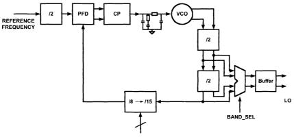
Fig.8. Architecture of the synthesizer.
