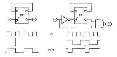
Fig. 10. Improved PSRR design of a divide-by-2 block.
