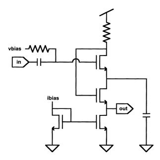
Fig.3. LNA topology that re-uses the current.
