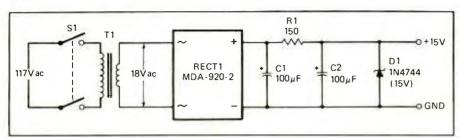
Fig. 2. Power for the Sprinkler Controller is obtained from the ac line.
