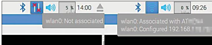
Figure 3. Before (left) and after (right). The Zero W should link up to the WLAN following configuration. Frequently you'll see additional information when you move the mouse over the symbols.
