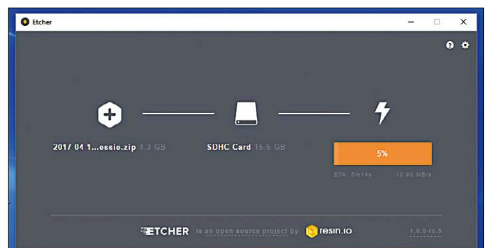
Figure 1. Etcher is an SD Card burning tool for loading the Raspbian image.
