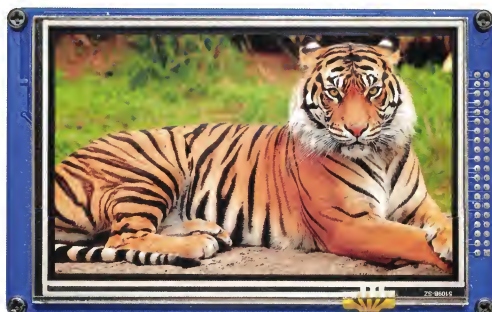
When using an LCD panel that has an SSD1963 controller, the Micromite Plus can display 800x480 pixels in true (24 bit) colour. This image of a tiger demonstrates the resolution and colour range.
