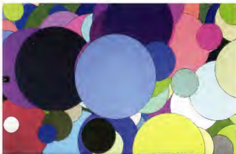
Fig.6: this is the display that you will see on the LCD when the command GUI TEST LCDPANEL is used. The display is animated with the circles being rapidly drawn on top of each other.
