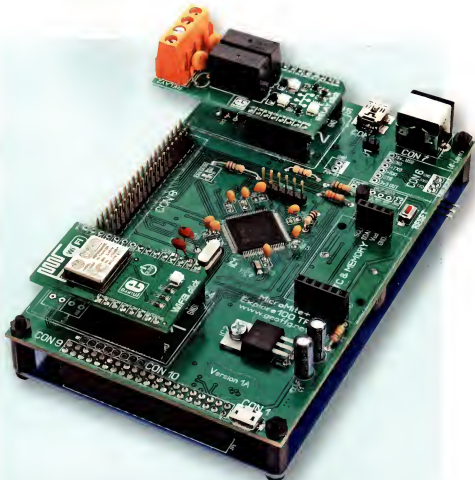
The Explore 100 has two sockets for mikroBUS-compatible Click boards. This is a standard developed by the European company MikroElektronika and covers a wide range of plug-in modules, including Ethernet, Bluetooth, WiFi and GPS modules – perfect for adding extra functions to the Explore 100. A WiFi board and a relay board are shown connected here
