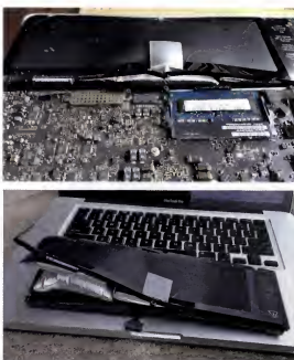
These photos show the battery as it appeared inside the case (top) and after it had been removed from the case. It had swelled enough to distort the chassis and the back.
