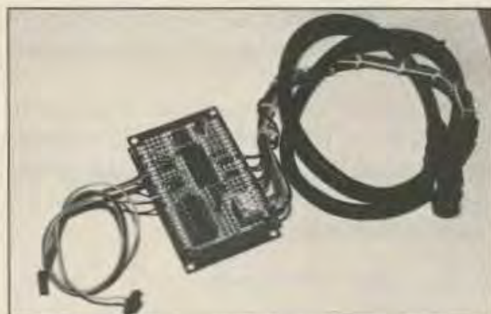
The adapter and cable that plugs into the Apple motherboard and an the IBM monitor.
