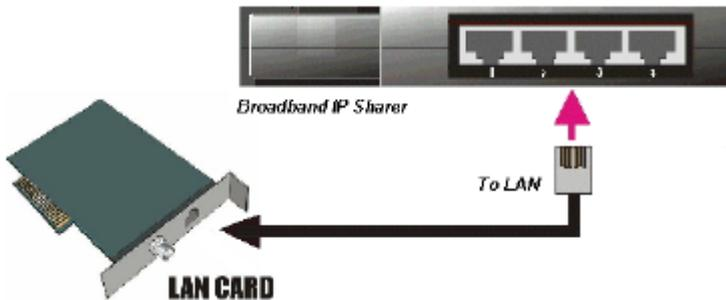
Figure 2-5 Setup of LAN connections for this product.
