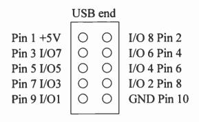
Figure 2.3 USB I/O 24 Port Connector pin configuration
