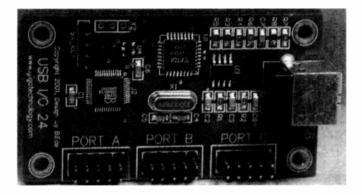
Figure 2.2 The USB I/O 24 module
