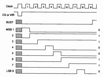
Figure 7.2 Successive approximation ADC waveforms
