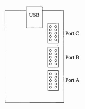
Figure 2.4 USB I/O 24 port layout
