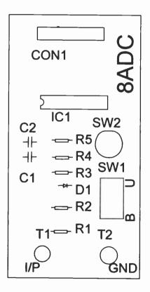
Figure A4.4 The 8ADC board component layout
