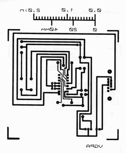
Figure A6.5 The VGPA PCB (Track side view)
