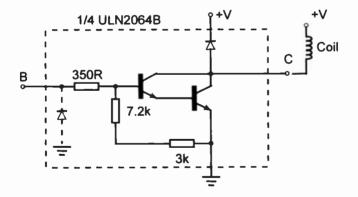
Figure A2.1 Circuit configuration for an individual stage
