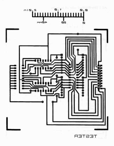
Figure A1.3 The User Port Tester PCB (Track side view)
