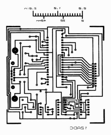
Figure A5.3 The 12ADC board PCB (Track side view)
