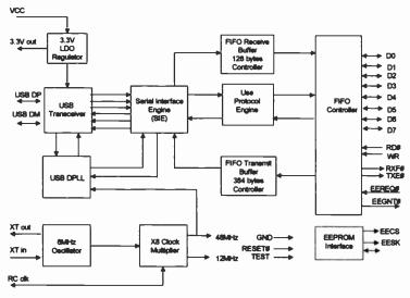
Figure 2.1 FT8U245 Block Diagram (Simplified)
