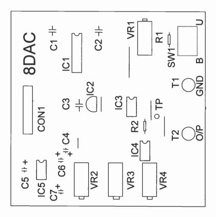
Figure A3.4 The 8DAC board component layout
