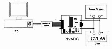
Figure 8.8 The 12ADC circuit layout
