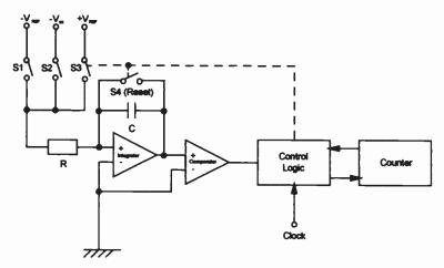
Figure 8.1 A dual-ramp integrating ADC
