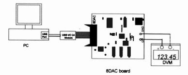
Figure 6.4 The 8DAC test circuit
