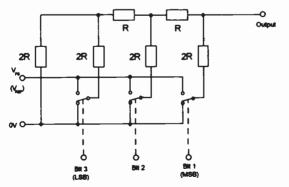
Figure 6.1 R-2R ladder DAC circuit
