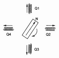
Figure 5.1 Permanent magnet stepper motor
