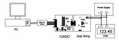
Figure 8.10 The 12ADC and VGPA circuit layout
