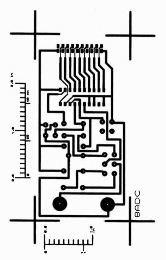
Figure A4.2 The 8ADC board PCB (Component side view)
