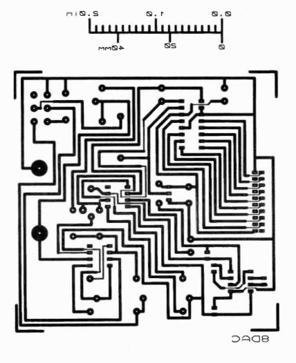
Figure A3.3 The 8DAC board PCB (Track side view)
