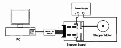
Figure 5.3 Stepper motor connections to the Stepper board
