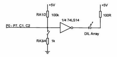
Figure A1.1 One LED driver circuit
