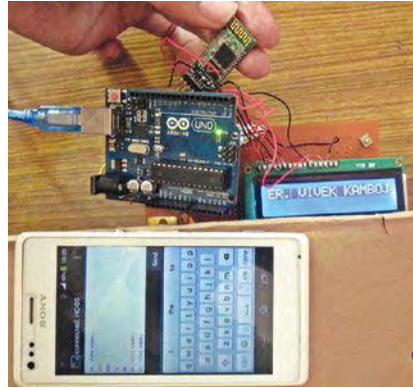
Fig. 2: Author's prototype of Arduino based programmable digital data display
