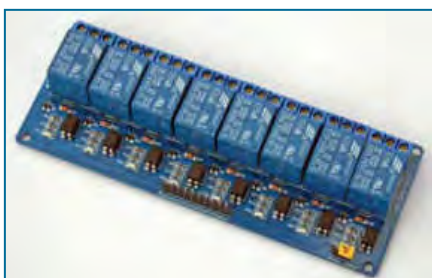
Fig. 2.9. An eight-channel relay interface board
