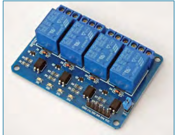
Fig.2.5. A four-channel relay interface board
