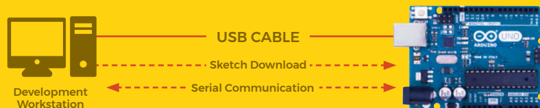
Figure 1 ◆ Arduino development architecture
