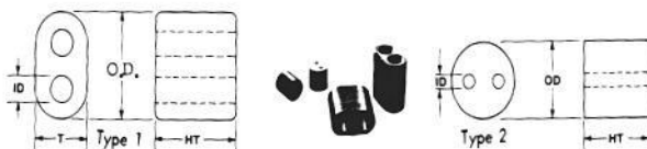
Dimensions in inches; A_L value in mh/1000 turns based on hole to hole winding
