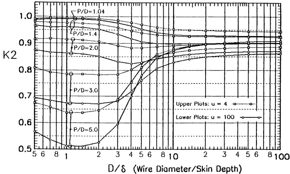
Fig. 7 Core Proximity Correction Factor  $K_2$
