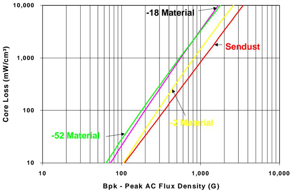
Figure 6: Core Loss vs. Bpk – 100 kHz
