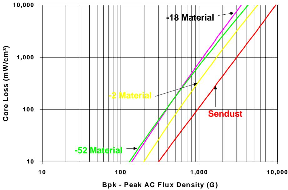
Figure 5: Core Loss vs. Bpk – 25 kHz
