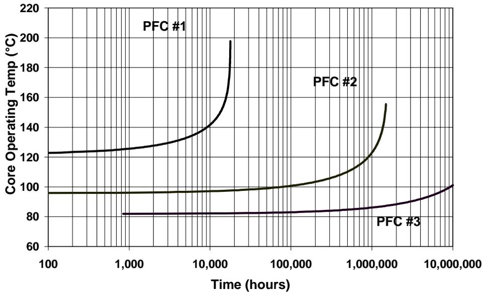
Figure 16: Core Operating Temperature vs. Time – PFC Designs
