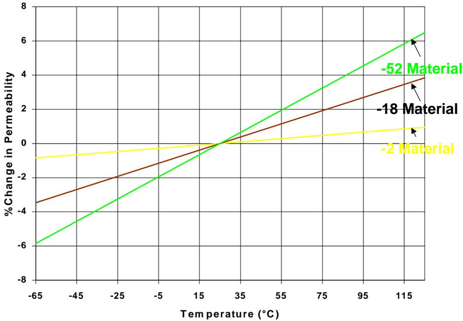
Figure 12: %Change in Permeability vs. Temperature – Iron Powder
