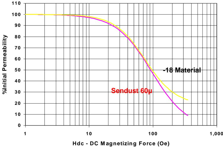
Figure 2: %Initial Permeability vs. H<sub>dc</sub>
