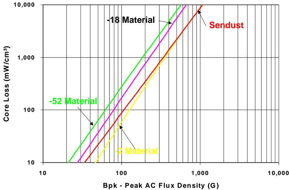
Figure 7: Core Loss vs. Bpk – 500 kHz
