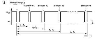
can be seen, overlaps in the pulse durations can occur in case of large differences between the temperatures of the individual sensors (e.g. sensor *n* at + 125 °C, sensor *n* + 1 at -40 °C). To the extent that such an unlikely situation can arise, it may be necessary to omit one of the timer regions, which would mean that the maximum number of sensors connected to a single line would be reduced to seven or six.
