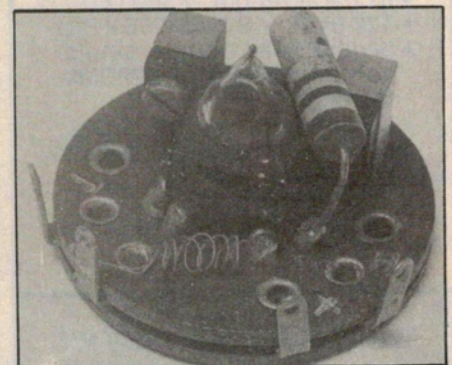
Fig.4: A small vacuum-enclosed thermocouple and load resistor combination, of the type used to measure RF power.
