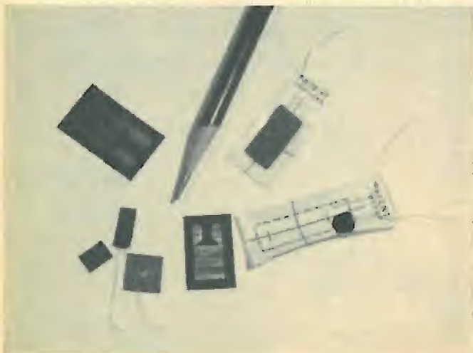
Fig. 3. These are examples of etched-foil and wire strain gages.
