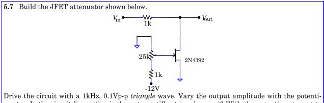
Drive the circuit with a 1kHz, 0.1Vp-p *triangle* wave. Vary the output amplitude with the potentiometer. Is the circuit linear (i.e. is the output still a triangle wave)? With the potentiometer set to produce a signal <sup>3</sup>/<sub>4</sub> as large as the input, what is the largest input signal passed relatively undistorted?
