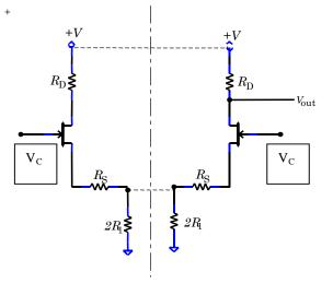
Since the transistors are identical, and since a common mode drive impresses the same signal on both transistors, both halves of the circuit will behave identically. Thus the common mode gain will be given by Eq. (1):
