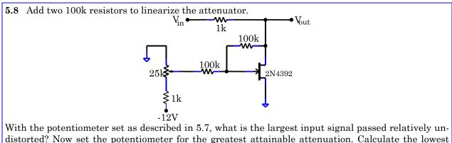
possible JFET drain-source resistance corresponding to this setting.
