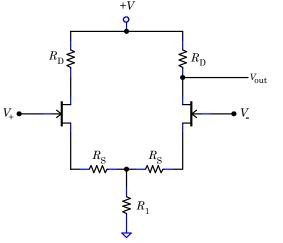
The amplifier's low common mode gain is immediately apparent by redrawing the circuit below:
