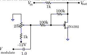
Add in a 1kHz 1Vp-p sine wave from another wave generator to the potentiometer signal through the  $V_{\text{modulate}}$  input. Set the potentiometer so that the carrier is modulated by the 1kHz wave. Sketch Vout.
