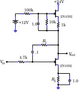
Aim for a feedback controlled gain of approximately 40.
