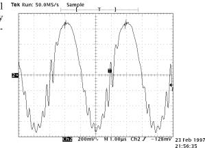
Touching the circuit, or even waving your hand near the circuit, can either accentuate or suppress the os-
