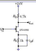
What is the gain now, experimentally, and theoretically? Is it frequency dependent? Why does the capacitor increase the gain? Is it as temperature dependent as the circuit in 5.3?
