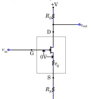
The equivalent small signal circuit for the amplifier is shown to the left and is most easily understood by remembering that the current in a source follower is given by  $V_{\text{in}}^{\bullet}$
