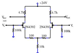
Leaving the  $V_{-}$  input attached only to its 100k resistor, drive the  $V_{+}$  input with a 1kHz, 0.1Vp-p sine wave. Measure the amplitude and phase of the output signal  $V_{out}$ . Look at  $V_{invout}$ ; what is the signal there? Reverse the setup; drive the  $V_{-}$  input. What are the amplitude and phase at  $V_{out}$ ? What about at  $V_{invout}$ ?
