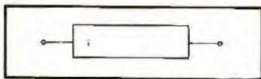
Fig. 3. A piece of intrinsic germanium with two leads, one at either end, like a common resistor. It can be used as a small photocell.
