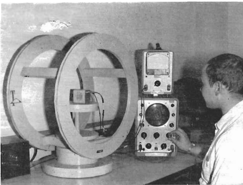
Magnetic shielding test setup using the Helmholtz structure.
