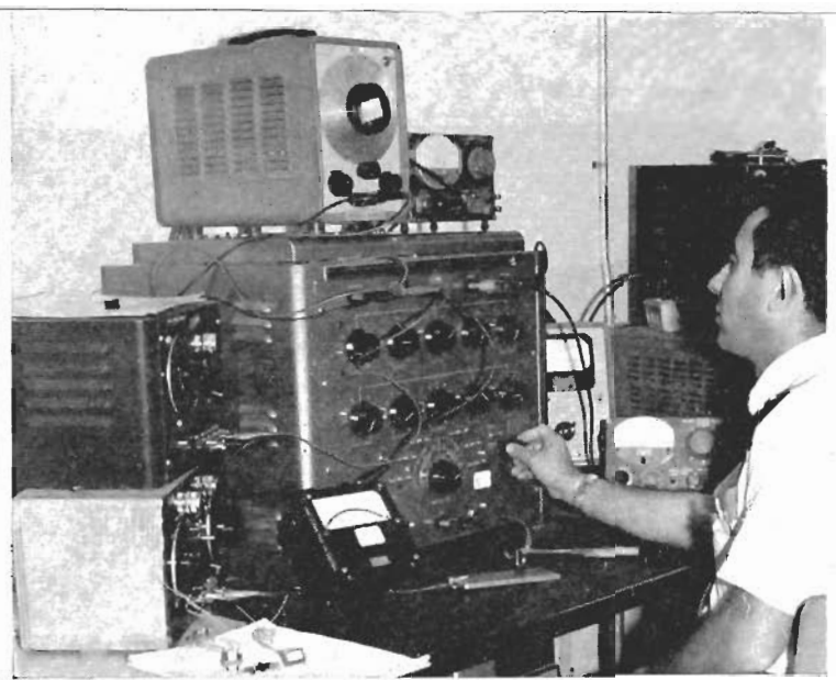
Test station for checking power chokes on inductance bridge.
