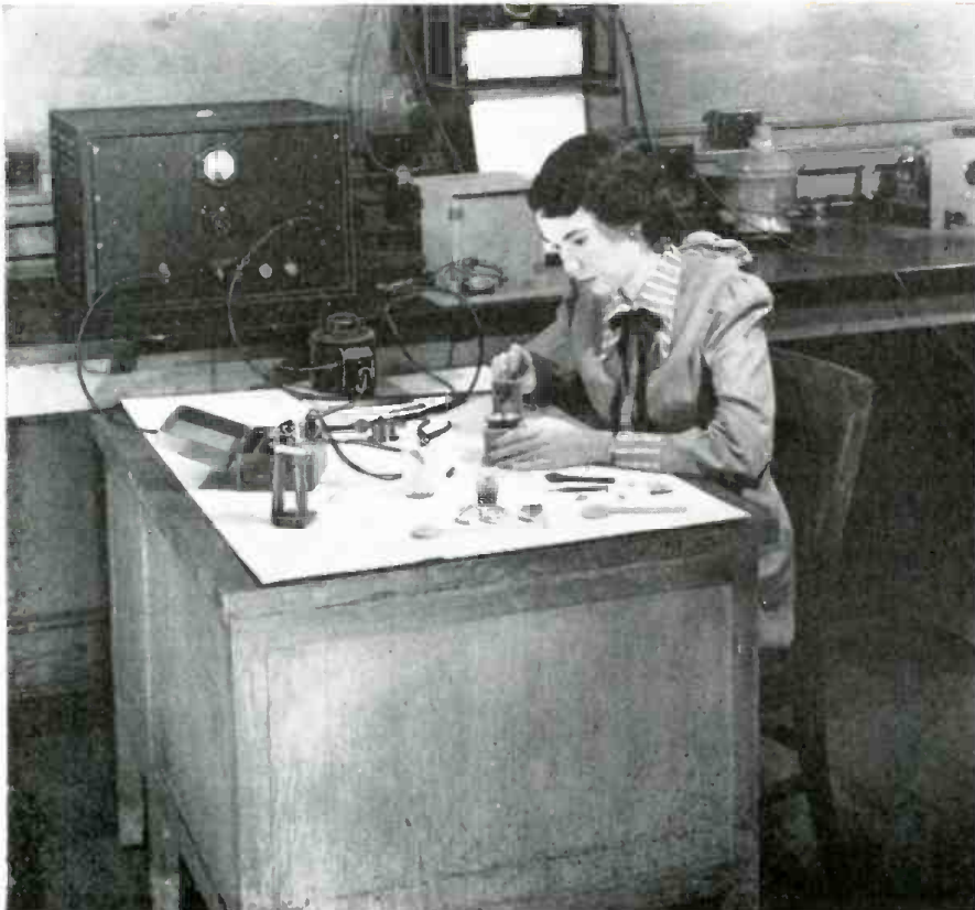
The author's sister engaged in removing from the mold a new electret just out of the oven.
