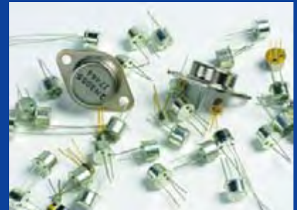
Switching transistors and power transistors from a Bargain Lot. The only thing you have to do is research the type codes to deduct the electrical functionality. Do not be afraid of a BCX863ABC. Avoid unlabelled devices.
