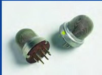
Sensors are in great demand simply because they are specialist components and expensive to buy as new items from manufacturers. Don't tell the seller — these two Figaro gas sensors are definitely a rare find.
