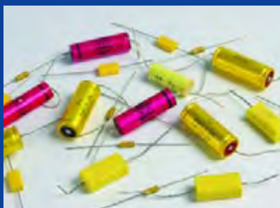
High voltage solid capacitors look bulky and dated in this day and age of low-voltage miniature portable equipment. For supply decoupling purposes, the value is not terribly important, so why not use that 0.068µF / 250V block capacitor?
