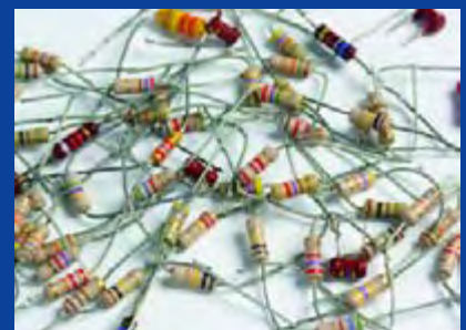
While most publications including Elektor now seem to assume everyone's on 1% metal film, there are still a number of good reasons to have a small stock of carbon resistors. For one thing, you can read the value in the blink of an eye!
