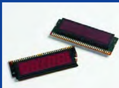
Displays are a source of hot debates and a lot of research because the manufacturer is never known so no-one ever seems to know the pin functions. These two beauties contain LED elements and were carefully salvaged from a 1980s alarm clock.
