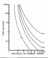
super time-lag (TT) fuse. Intermediate speeds are obtained with the other classes which were referred to in the penultimate paragraph of my article. These differences are achieved by specially designed fuse elements and the wide choice in operating speeds should cover the requirements of most users.
