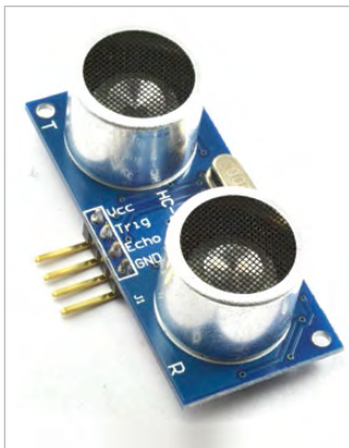
Left The HC-SR04 Ultrasonic Rangefinder. Cheap-as-chips sonar
