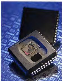
Bosch solid state MEMS gyroscope and low g-force sensor for rollover detection.
