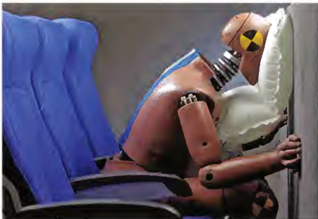
Amsafe seat belt airbag in crash simulation with aircraft bulkhead in front of passenger.
