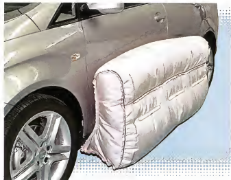
(Above): 2013 Volvo V40 showing pedestrian air bag which also raises the bonnet when activated.
