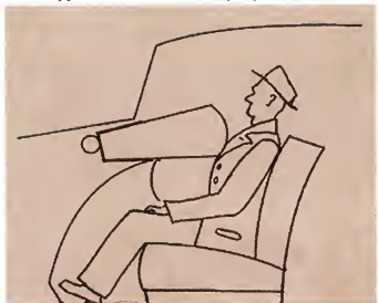
Drawing from German patent 896,312 of 1953 by Walter Linderer. It was filed on October 6th, 1951 and granted November 12th, 1953. Loosely translated into English, the title of the patent is "Facility for the protection of passengers against injuries in vehicle collisions".
