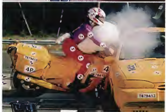
Test of early motorcycle airbag on a Norton Commander in a frontal collision with side of car. UK Transport Research Laboratory and Lotus Engineering, report published 1996.
