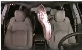
(Above): centre airbag to stop passengers hitting each other in the event of a side impact.
