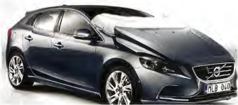
(Above): 2013 Volvo V40 showing pedestrian air bag which also raises the bonnet when activated.
