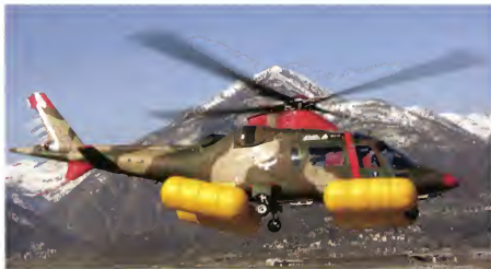
Aero Sekur external airbags on a helicopter. The system was showcased at the 2010 Farnborough International Airshow but does not appear to have been commercialised.
