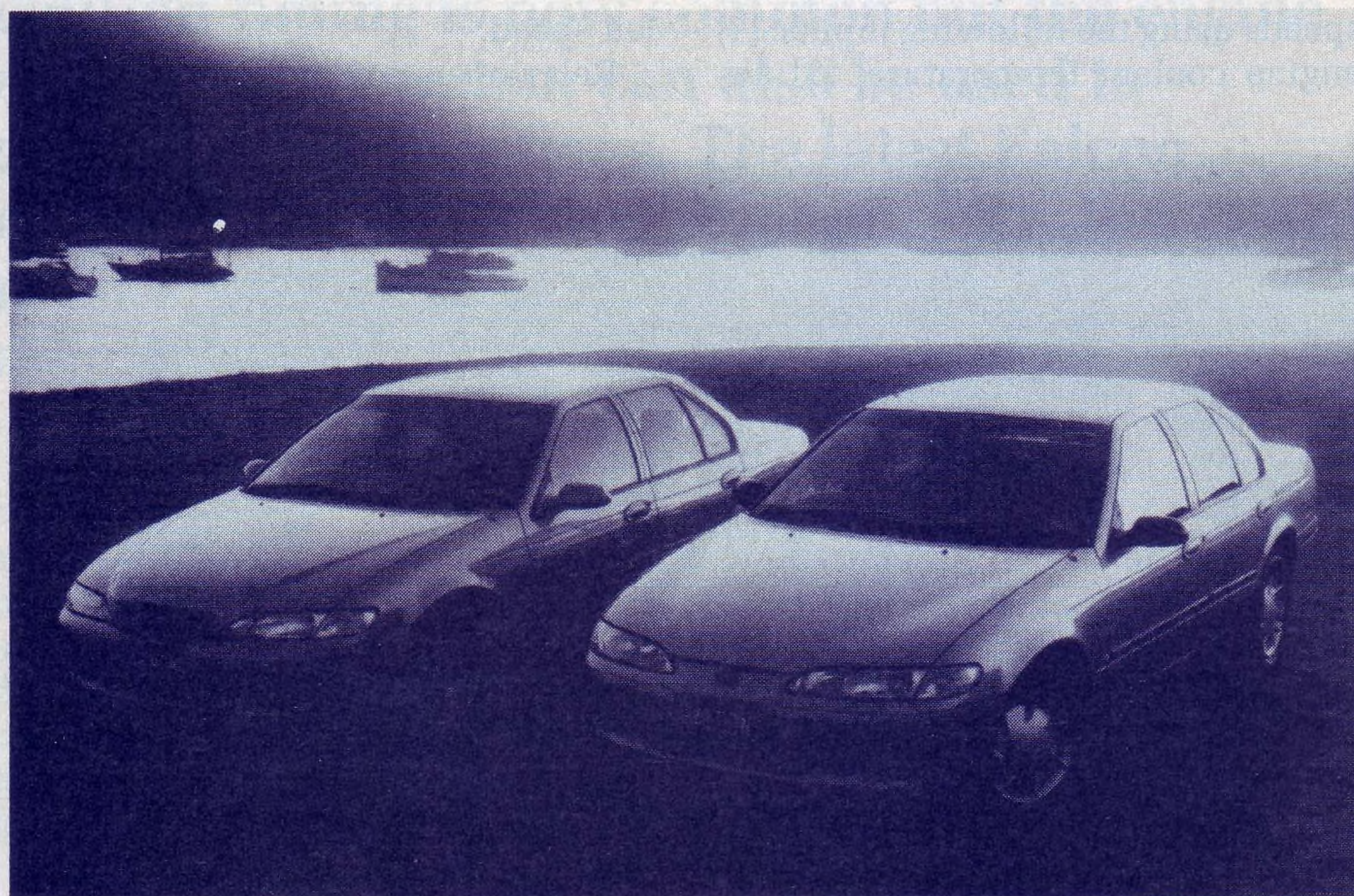
The bar across the under-bumper air intake on Fairmont models (left) needs to be precisely angled during manufacture so that it doesn't degrade cooling performance. The above-bumper grille is a dummy & is there for styling only!
