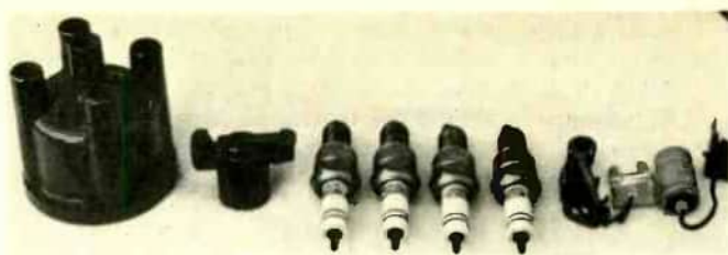
This is a typical ignition tune-up kit for a 4-cylinder car. From left to right: distributor cap, rotor, spark plugs, points, and condenser.
