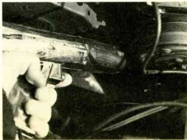
Use of the timing light allows you to freeze the action of the flywheel and read the timing adjustment. A decal under the hood will list number of degrees (either in BTDC or ATDC) to which pointer on the flywheel must point to on scale next to the flywheel. Timing is adjusted by rotating the distributor body.
