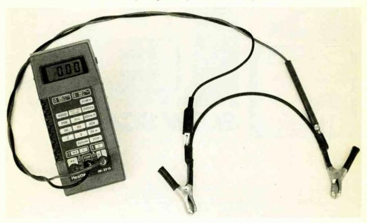
F YOU WANT to measure the large current from your car's alternator or starter, here are a few tricks on how to do it with your digital multimeter.
