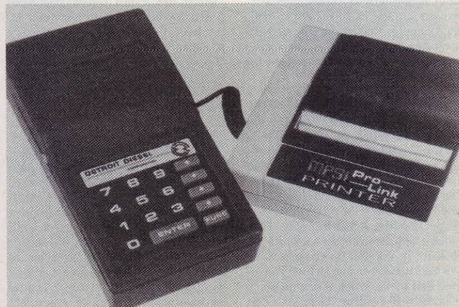
The Diagnostic Data Reader can be used to program factors such as the cruise control settings, vehicle ID number, engine power rating & vehicle speed limiting. It also can download engine faults logged in the ECM's memory.
