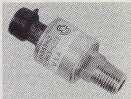
This sensor is designed specifically for fire truck operation & measures fire pump water pressure. The engine speed is then adjusted by the ECM to give a constant water pressure.
