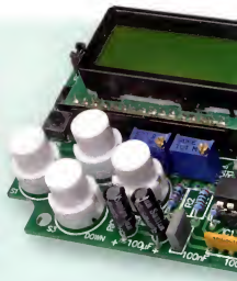
Fig.2: follow this parts layout diagram and the photo to build the PCB. The LCD module plugs into a 16-way pin header and is supported on two spacers. Make sure that all polarised parts are correctly orientated.
