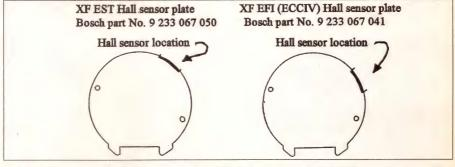
Auto Electronics (October 1996): In Fig.7, on page 45, the Hall Sensor plates for XF Falcon EST and EFI (EECIV) systems were unfortunately swapped. The corrected diagram is shown above.
