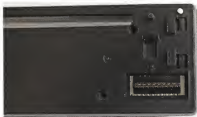
Fig.5 (above) shows the multi-way connector which is used to connect the front panel to the head unit.
