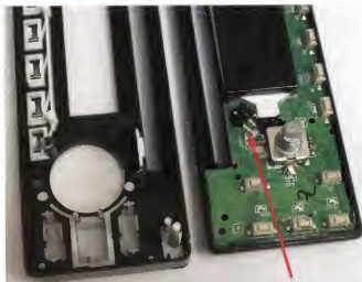
Fig.5 (above) shows the multi-way connector which is used to connect the front panel to the head unit.
