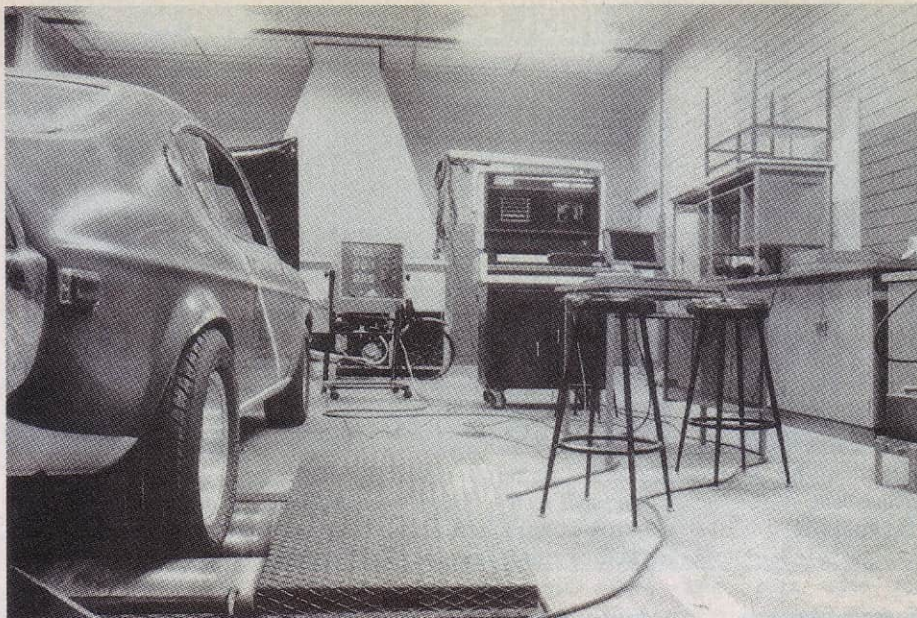
Chassis or engine dynamometers and exhaust gas analysers are required to set up programmable fuel injection ECUs.
