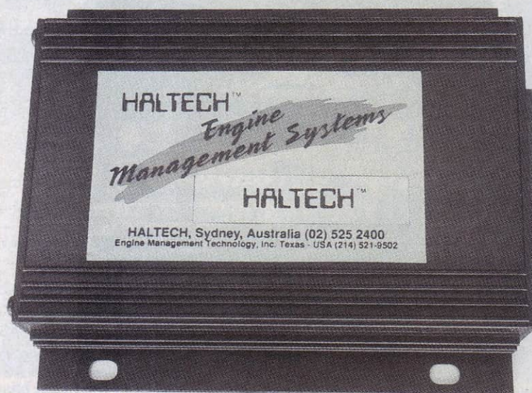
The Haltech engine management ECU. It can be programmed to compensate for coolant temperature, air temperature and the battery voltage, and has optional closed-loop oxygen sensor feedback control.
