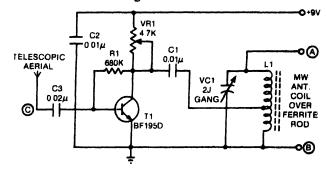
Assemble the unit on a small general-purpose veroboard. House it in a small plastic cabinet with the antenna coil L1 and the ferrite rod cemented to the side or back of the cabinet using an adhesive like araldite for best performance. Adjust coil L1 over the ferrite rod before cementing it on to the cabinet. The unit should be positioned parallel to the built-in antenna coil of the receiving set.
