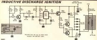
WITHOUT going into the controversy about the advantages of capacitor or inductive discharge ignition versus normal ignition, a circuit for inductive discharge ignition is presented here. It is a points assisted unit in which the coil load of 3-5 amps is removed to a switching transistor. Other features in the circuit are: rev limit. points bounce control, long dwell time, lower RF1 than a CD1 system
