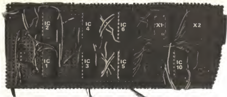
The author's Fuel Consumption Meter circuit was laid out on two pieces of Veroboard mounted one behind the other. Component layout is non-critical, and this photograph shows the basic arrangement of the counter section of the prototype unit.
