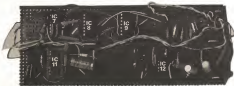
Interfacing section circuit board. Use Fig. 3 for interwiring. This board should be mounted so that the displays show through the front panel directly.
