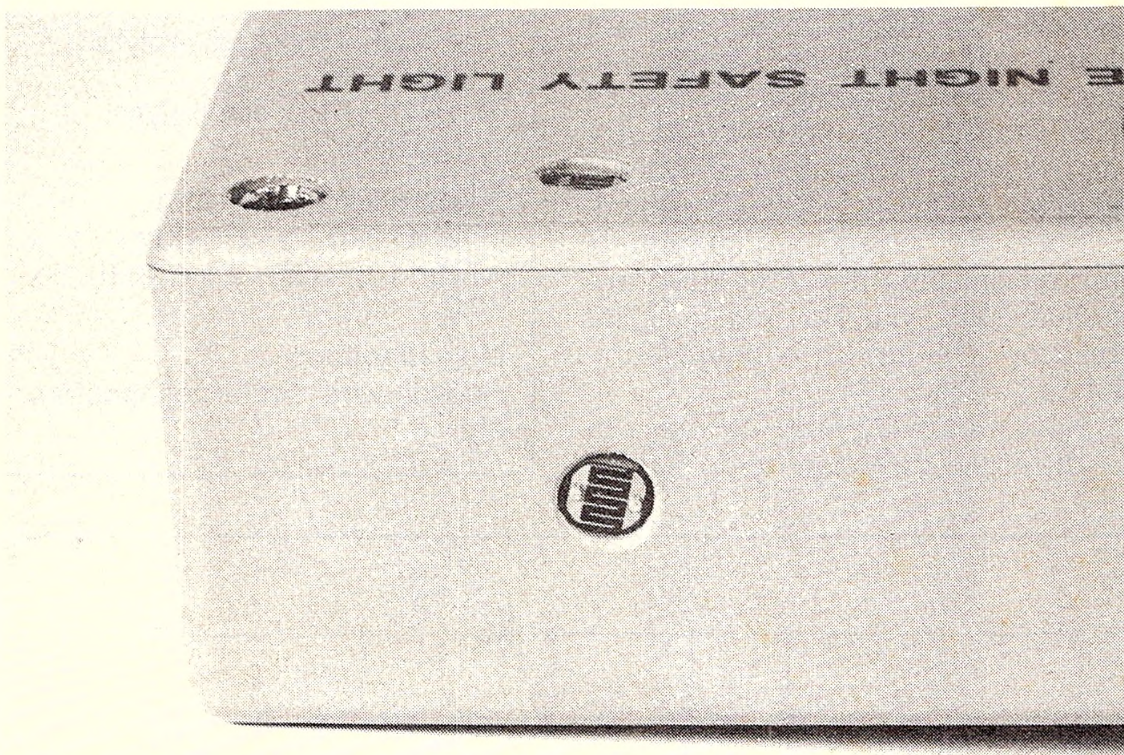
The two LDRs are simply pushed into small holes drilled through the lid and side of the case. Note how the top LDR sits below the surface of the lid so that it cannot pick up light from an approaching car's headlights.
