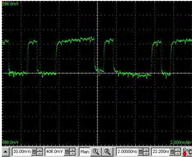
Figure 59 Random data stream showing minimum driver output of 0.8mA
