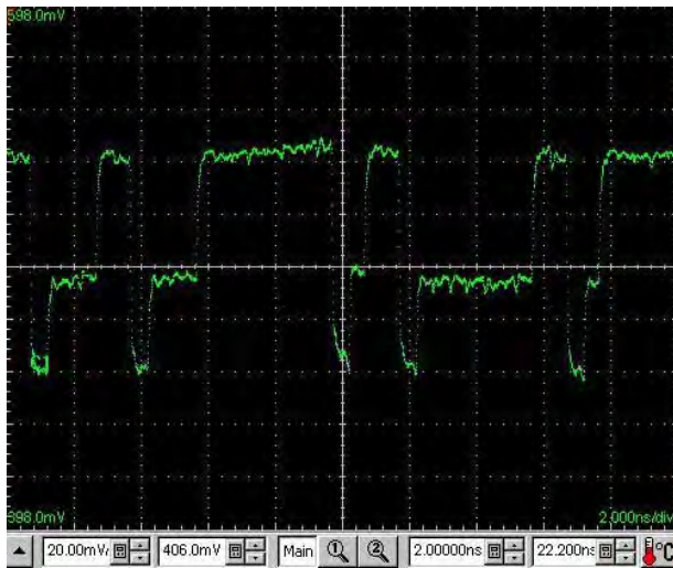
Figure 61 Random data stream showing the first half of tap 1 turned on and all others off
